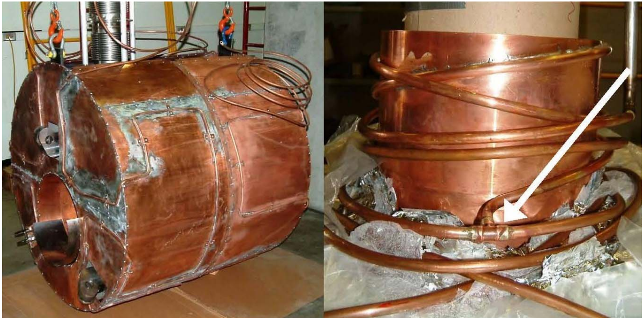
FIG. 13. Left: Outer heat shield around body of Big Sol (note: the chimney is not installed in this picture). Right: LN2 is fed from above and originally looped around the chimney before branching off to the body. The repair redirected the feed directly to the body as shown by the white arrow.
